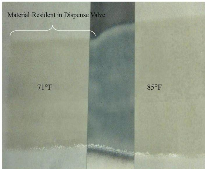
**FIGURE 5:** The effect of thermal loss on spray pattern
