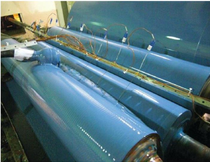
**FIGURE 7:** Measuring temperatures in a roll coating system
