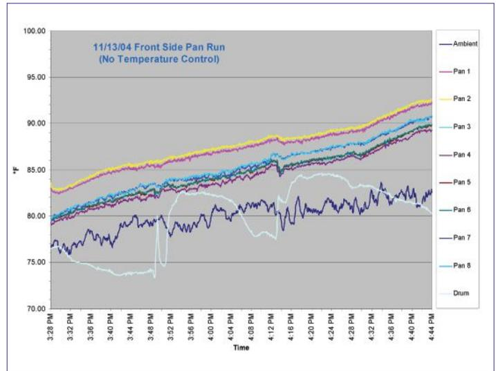
**FIGURE 8:** The effect of process friction on temperature<sup>1</sup>
