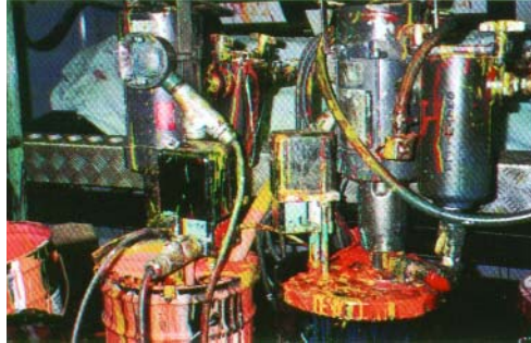
The M8BO measuring element, seen here jutting out of the 5-gal ink pail, is designed for easy cleaning. Even if ink is allowed to dry inside it overnight, the system can be disassembled and cleaned in two minutes.
